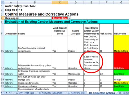
Figure 7: Aligning hazards/hazardous events with SANS 241 determinants to allow development of risk-based monitoring programme
